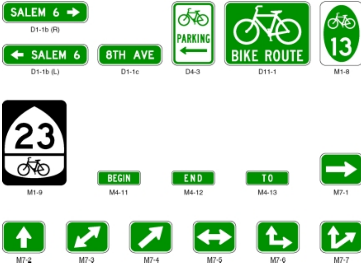
Figure 9B-4. Guide Signs for Bicycle Facilities
