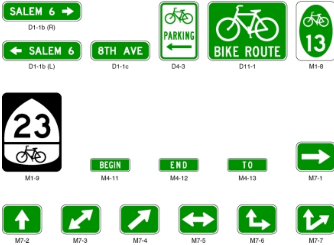
Figure 9B-4. Guide Signs for Bicycle Facilities
