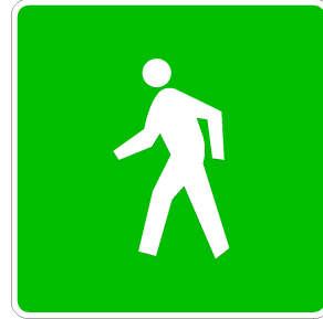
D11-2 450 x 450 mm (18 x 18 in) min. White symbol & border on green background
