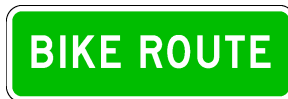
D11-1b 450 x 150 mm (18 x 6 in) min. White symbol & border on green background
